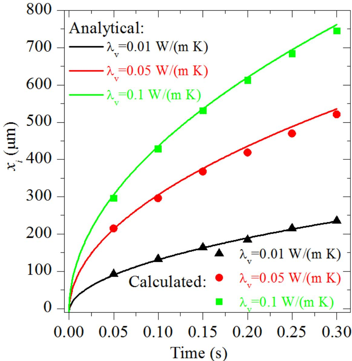
Vapor-liquid interface position  $x_i$  as a function of time for different values of  $\lambda_v$ :
