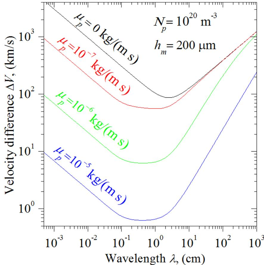
melt destabilization due to plasma viscosity effects with a slight shift in critical wavelength toward shorter waves
