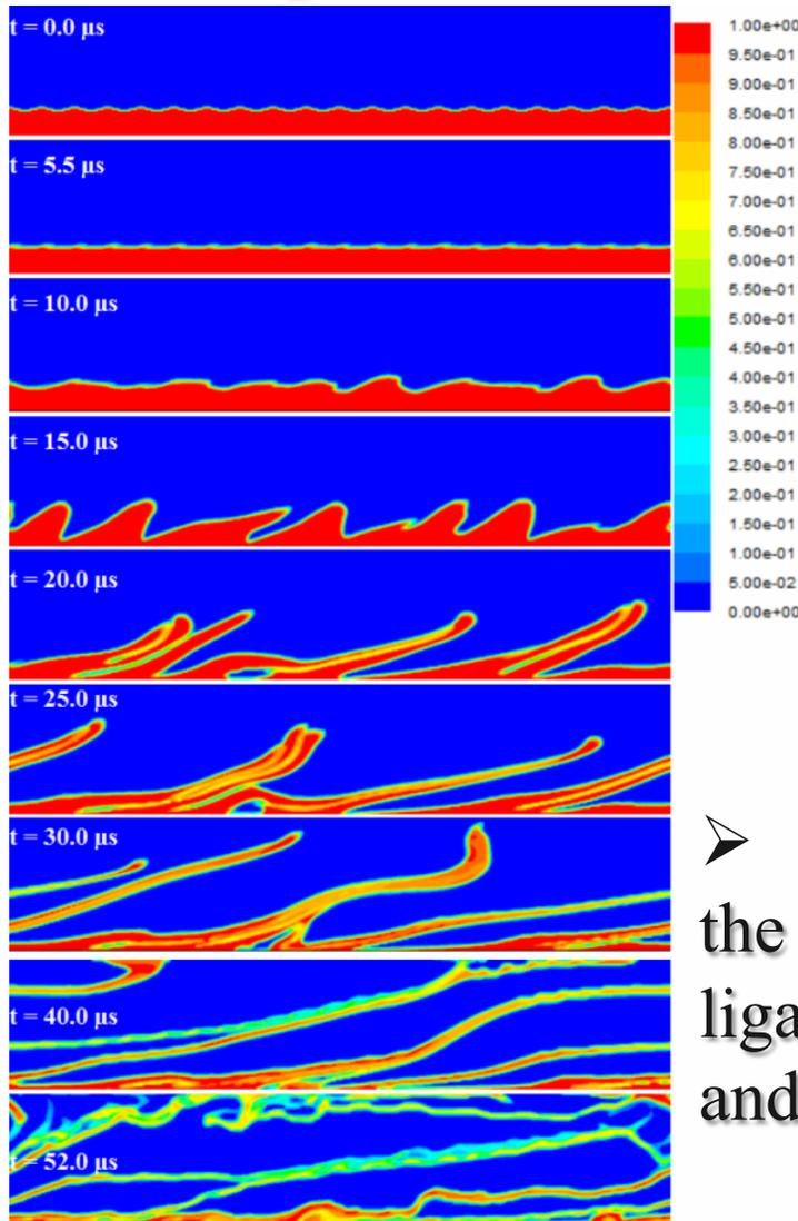
*Plasma-liquid tungsten interface perturbed with shorter wavelength,  $\sim 0.5$  mm*
