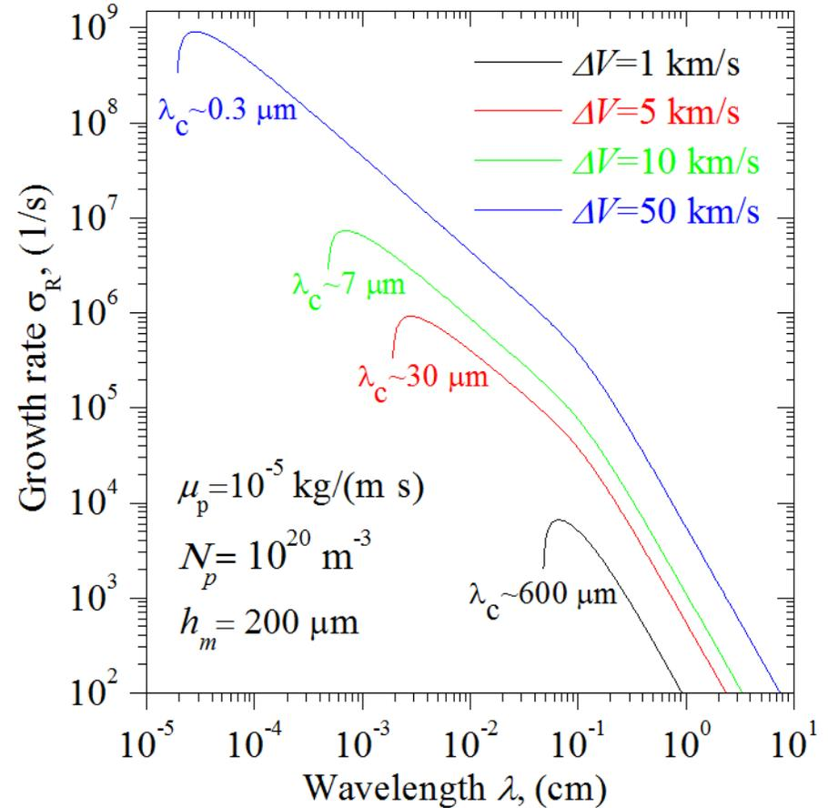
significant increase in growth rate of short waves (dangerous wavelengths) with increase in plasma velocity
