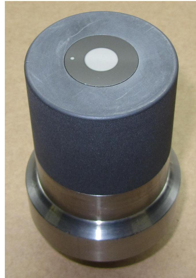
DiMES probe for 5/1/12; 1 cm and 1 mm Mo spots on carbon probe
