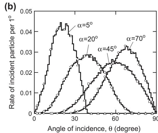
Angular distribution of incident H ions for shallow and perpendicular angle between B and surface
