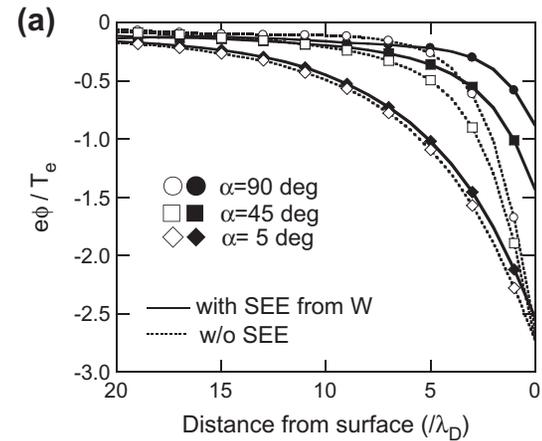
Potential distribution from a W surface for shallow and perpendicular angle between B and surface
