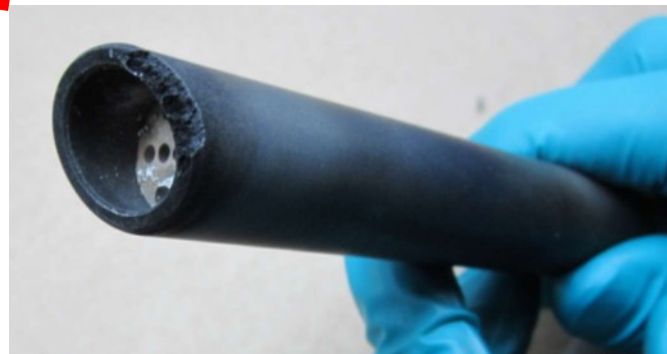
Damaged midplane probe head
