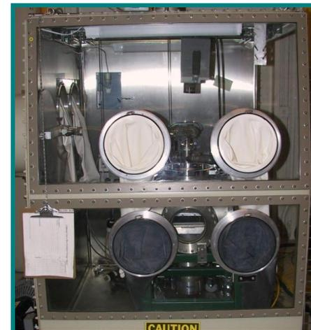
We use an argon glove box to transfer Li in an inert atmosphere.
