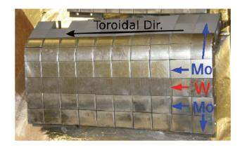
Toroidally symmetric tungsten tiles at/near outer divertor strike point. Exposed for  $\sim 10^3$  s at various plasma conditions.
