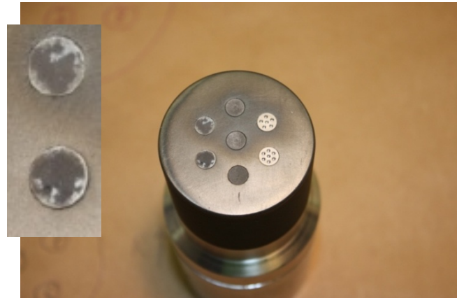
Loaded DiMES sample 2 Si-W, 3 graphite, 2 W buttons
