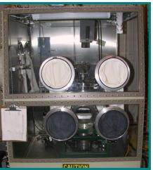
We use an argon glove box to transfer Li in an inert atmosphere.
